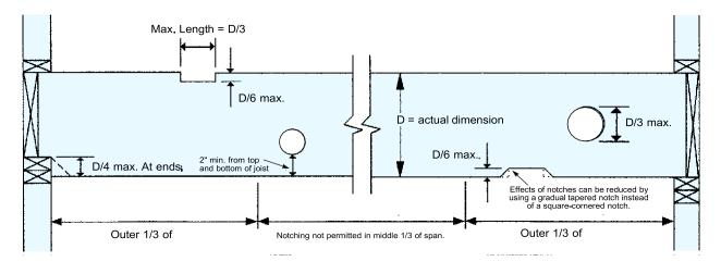
Fig. 2: Notches in 2x4 Studs
