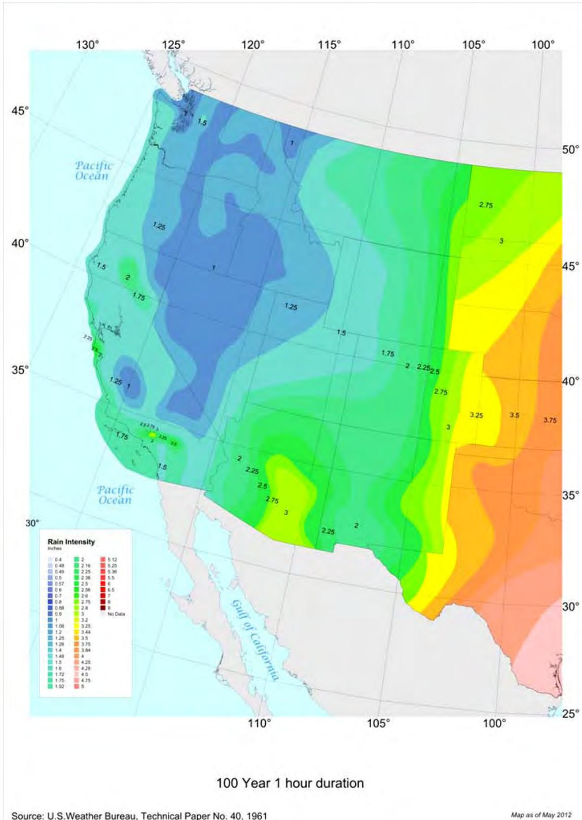
Fig. C5. 100-year, 60-minute Rainfall intensity (i) in inches per hour for the western United States (to convert to millimeters per hour multiply by 25.4)
