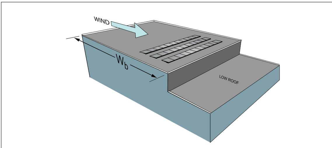
Fig. 2.6.2.3-5. Upwind fetch distance ( $W_b$ ) for leeward snow drift at low roof with solar panels on high roof
