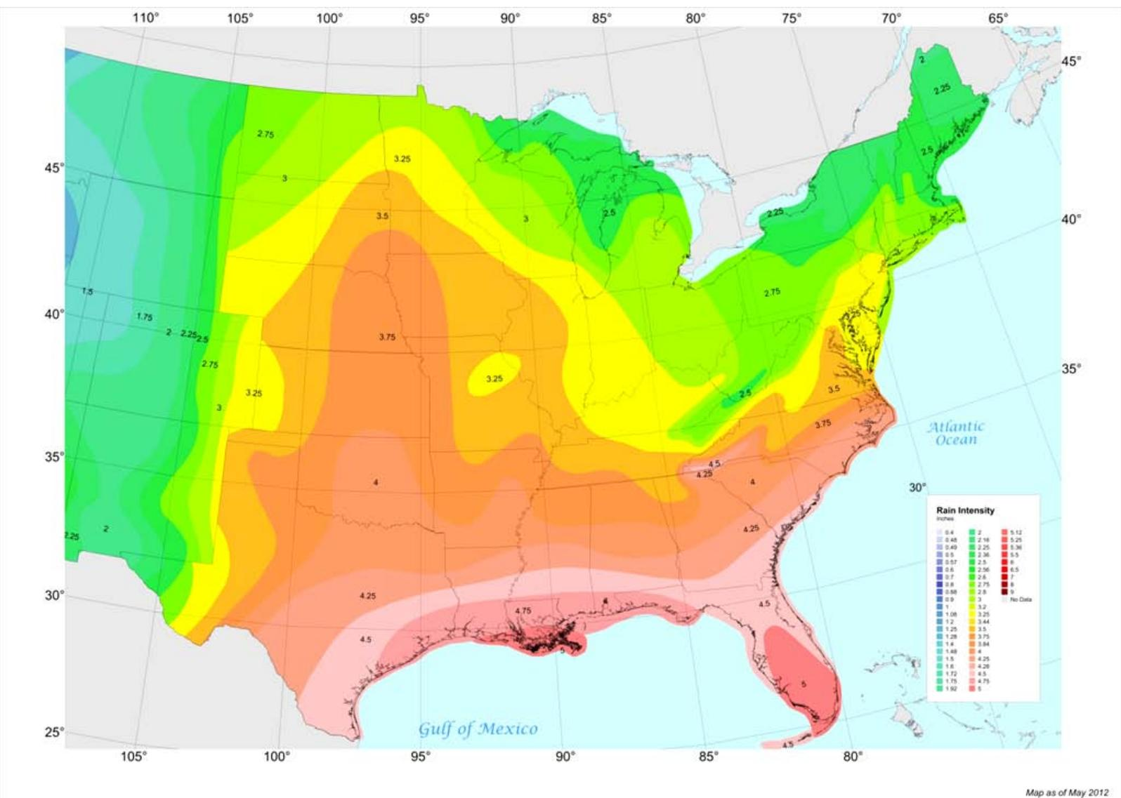
Fig. C6. 100-year, 60-minute Rainfall intensity (i) in inches per hour for the central and eastern United States (to convert to millimeters per hour multiply by 25.4)
