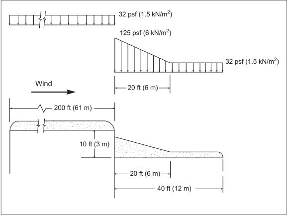
Fig. E.1-3. Design snow loads for Example 3 (Leeward Drifting)
