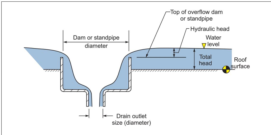
Fig. 2.5.4.1-2. Overflow (secondary) roof drain with hydraulic head and total head (debris guard not shown for clarity)
