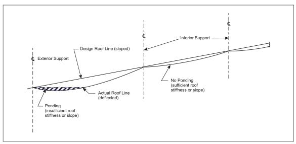
Fig. 2.5.4.1-4. Sloped roof with roof edge drainage
