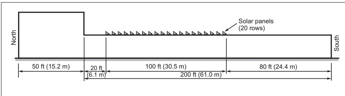
Fig. E.3-2 Elevation view of roof with solar panels
