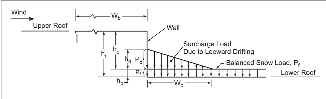
Fig. 2.4.5.1-1. (To be used with Table 2.4.5.1) Leeward snow loads for lower roofs
