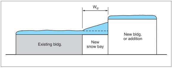
Fig. 2.4.6. New snow bay to prevent drift loading on an existing roof
