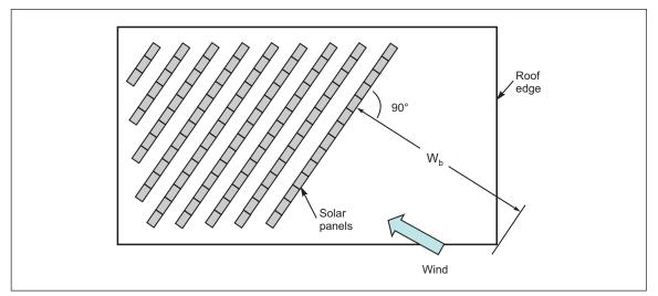
Fig. 2.6.2.3-15. Upwind fetch distance ( $W_{b}$ ) for snow drift at closely spaced skewed rows of solar panels
