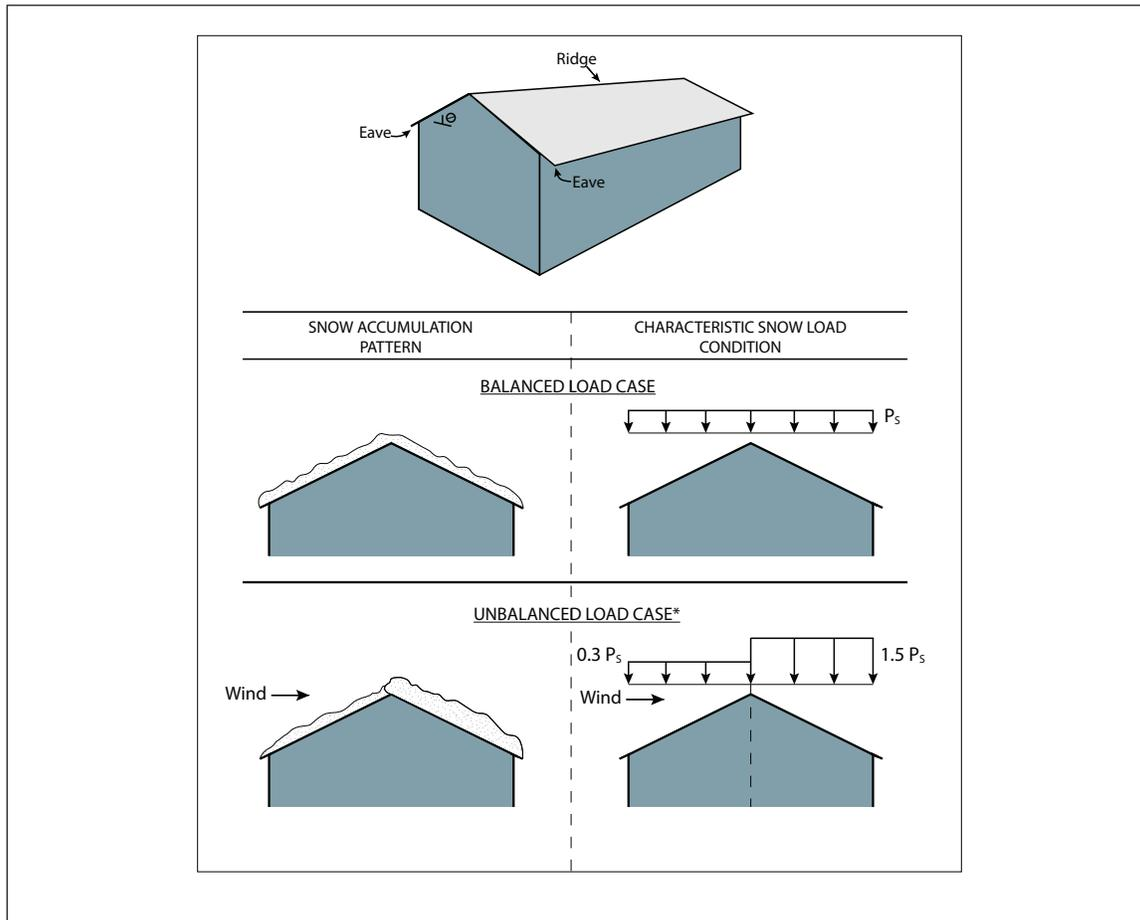
Fig. 2.4.4.3. Snow loads for hip and gable roofs
