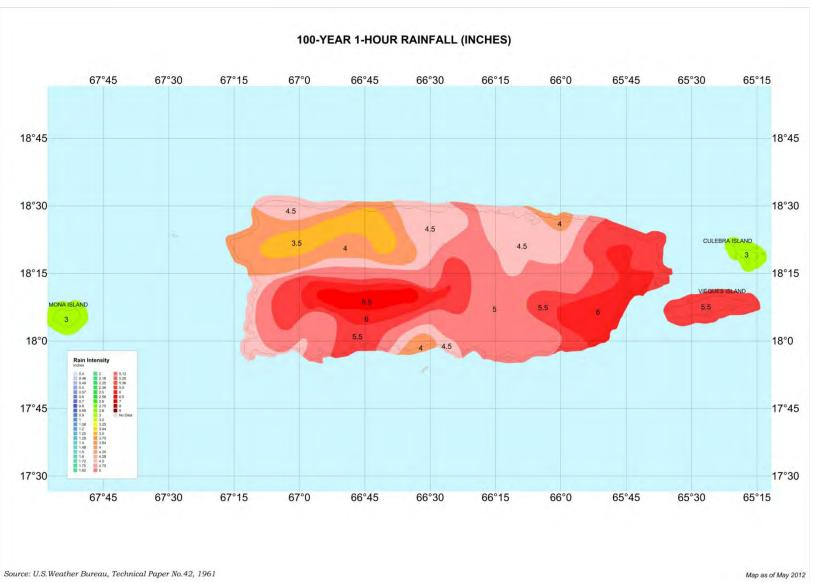
Fig. C7. Rainfall intensity (i) in inches per hour for Puerto Rico (to convert to millimeters per hour multiply by 25.4)
