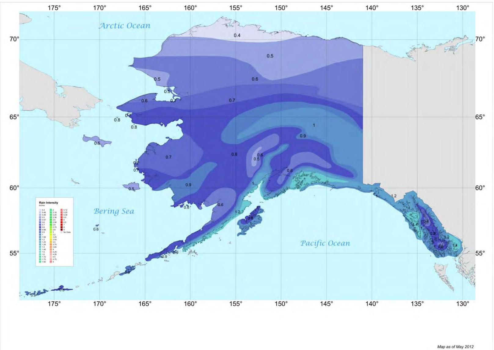
Fig. C9. 100-year, 60-minute Rainfall intensity (i) in inches per hour for Alaska (to convert to millimeters per hour multiply by 25.4).
