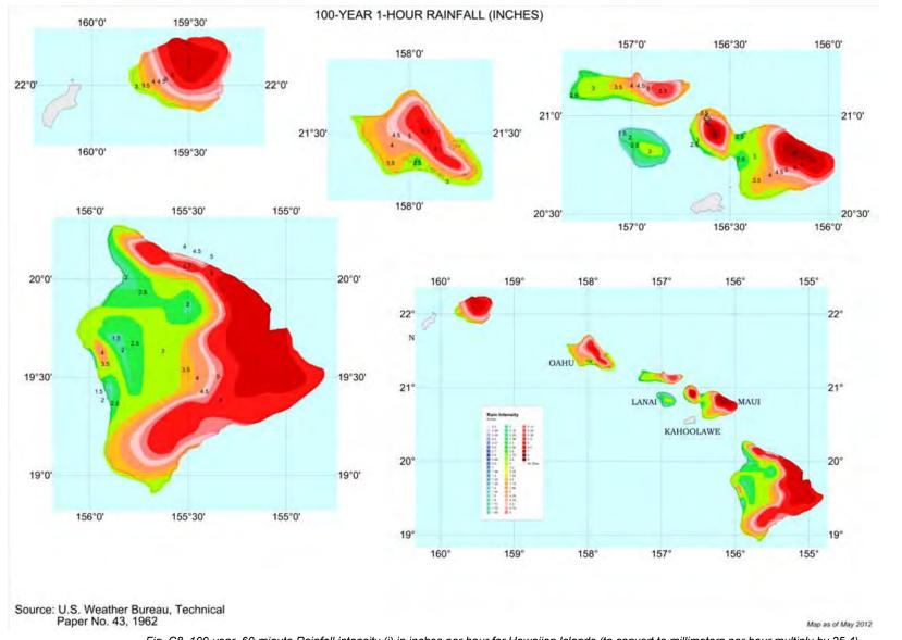
Fig. C8. 100-year, 60-minute Rainfall intensity (i) in inches per hour for Hawaiian Islands (to convert to millimeters per hour multiply by 25.4)
