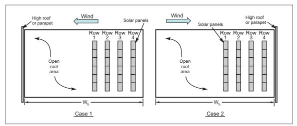
Fig. 2.6.2.3-8. *W<sub>b</sub>* for snow drift at parapets, roof projections, or high roof walls for flush-mounted solar panels, widelyspaced titled solar panels, and tilted solar panels with less than significant height
