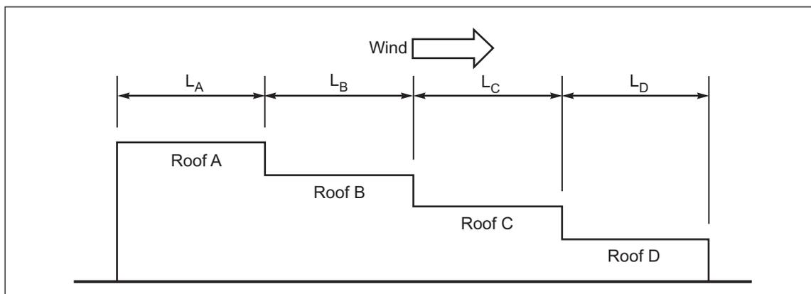
Fig. 2.4.5.1-3.  $W_b$  for leeward snow drift at multiple roofs steps
