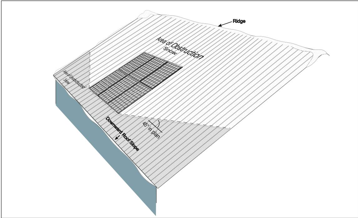
Fig. 2.6.2.3-2. Obstructed portions of sloped roofs
