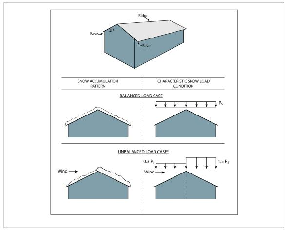
Fig. 2.4.4.3. Snow loads for hip and gable roofs
