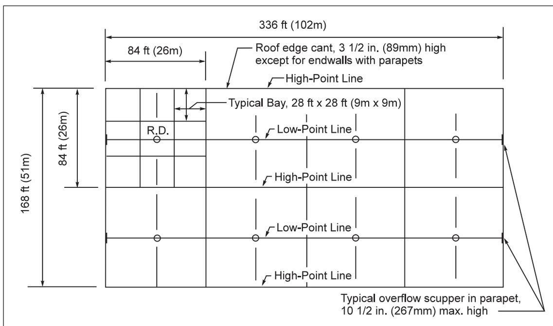
Fig. E.2-1 Sloped roof plan for Example 5
