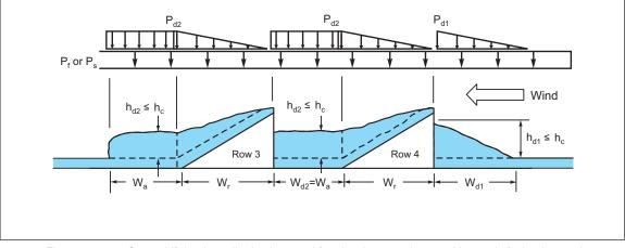
Fig. 2.6.2.3-13. Snow drift loads at tilted solar panel for closely spaced rows with panels facing leeward
