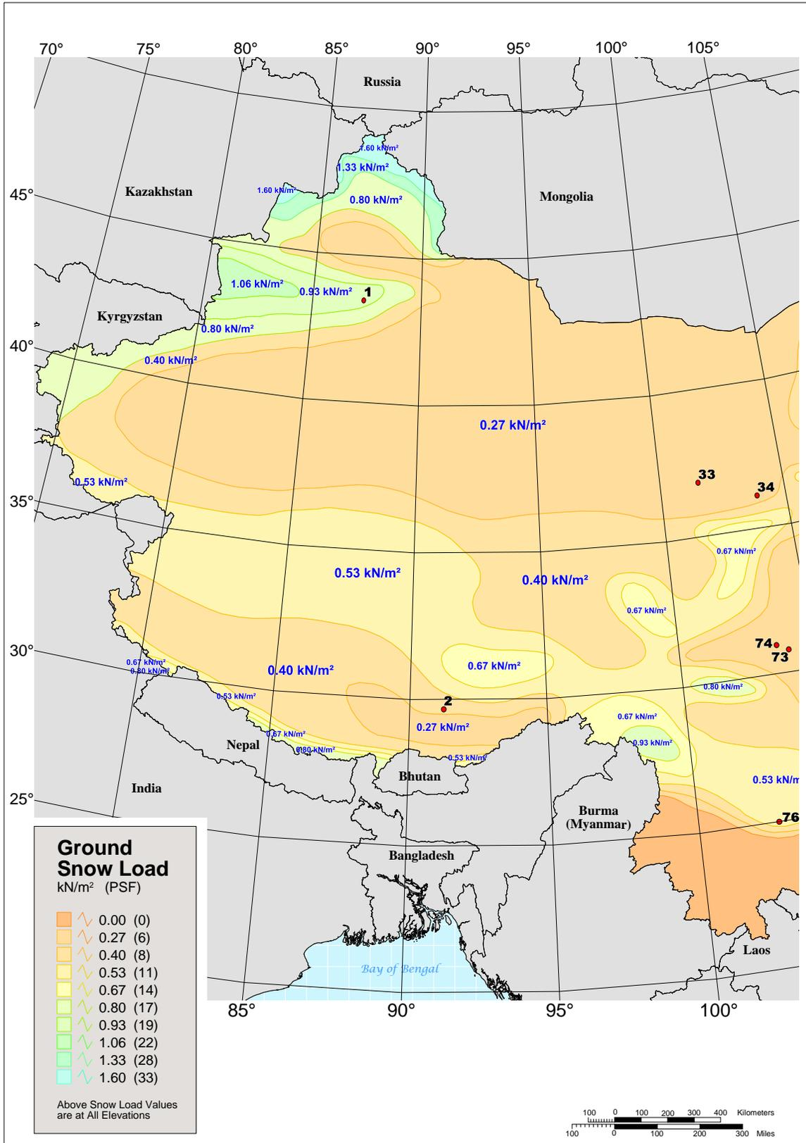
Fig. C3. Ground snow load ( $P_g$ ) in  $kN/m^2$  for Western China
