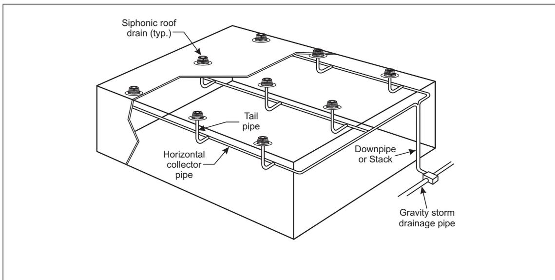
Fig. 2.5.4.2-1. Diagram of siphonic roof drain system
