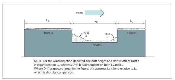
Fig. 2.4.5.1-6. Windward and leeward drifing at a roof pocket
