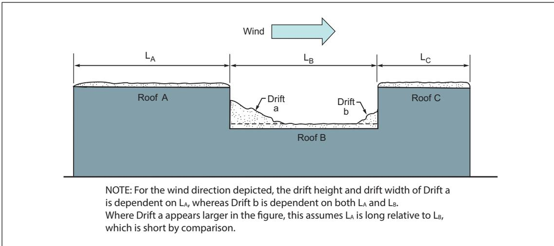
Fig. 2.4.5.1-6. Windward and leeward drifting at a roof pocket
