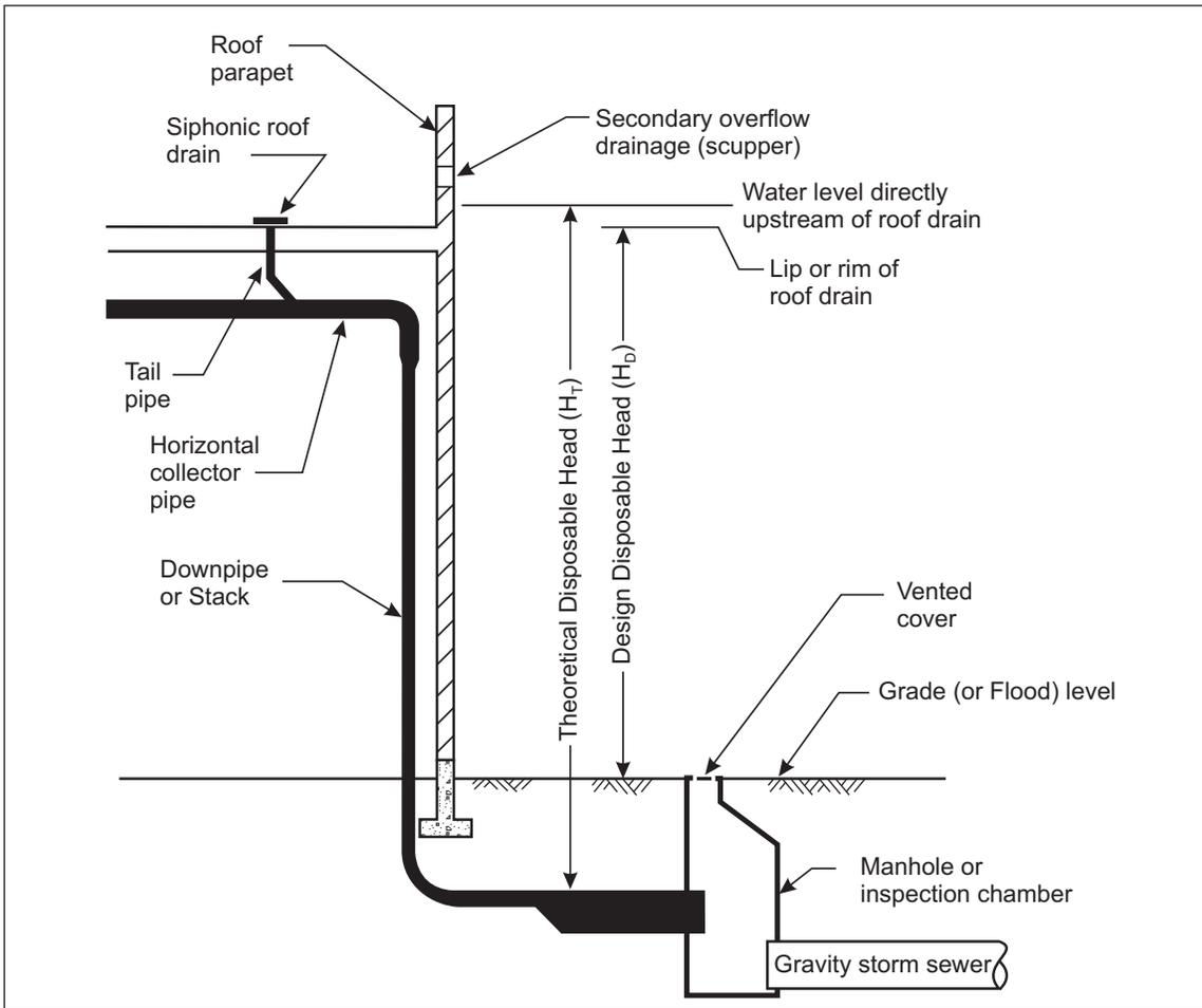
Fig. 2.5.4.2-2. Elevation view of siphonic system and disposable (available) head
