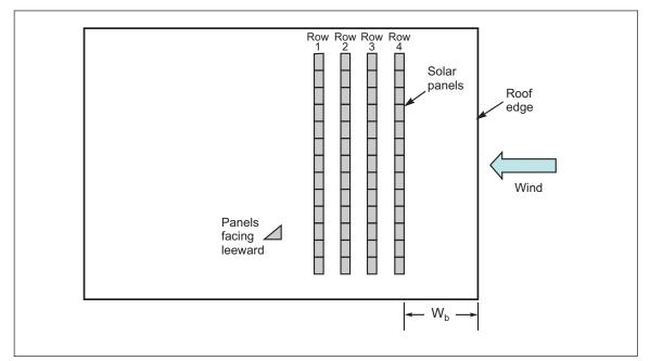
Fig. 2.6.2.3-14. Upwind fetch distance (W<sub>b</sub>) for snow drift at multiple rows of closely spaced tilted solar panels with panels facing leeward
