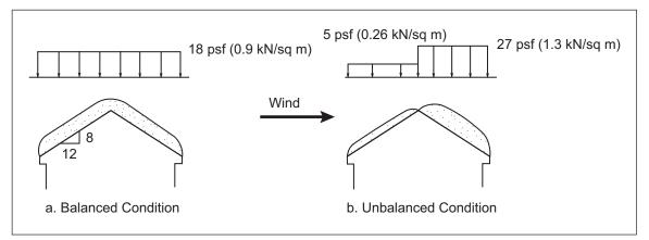
Fig. E.1-1. Design snow loads for Example 1
