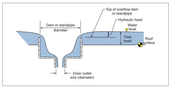
Fig. 2.5.4.1-2. Overflow (secondary) roof drain with hydraulic head and total head (debris guard not shown for clarity)
