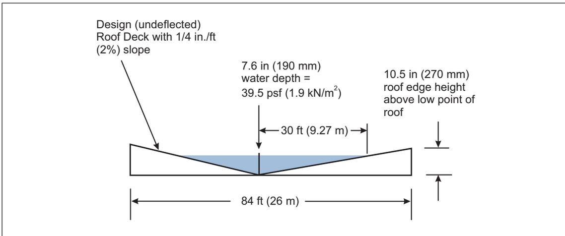
Fig. E.2-2 Sloped roof section for Example 5
