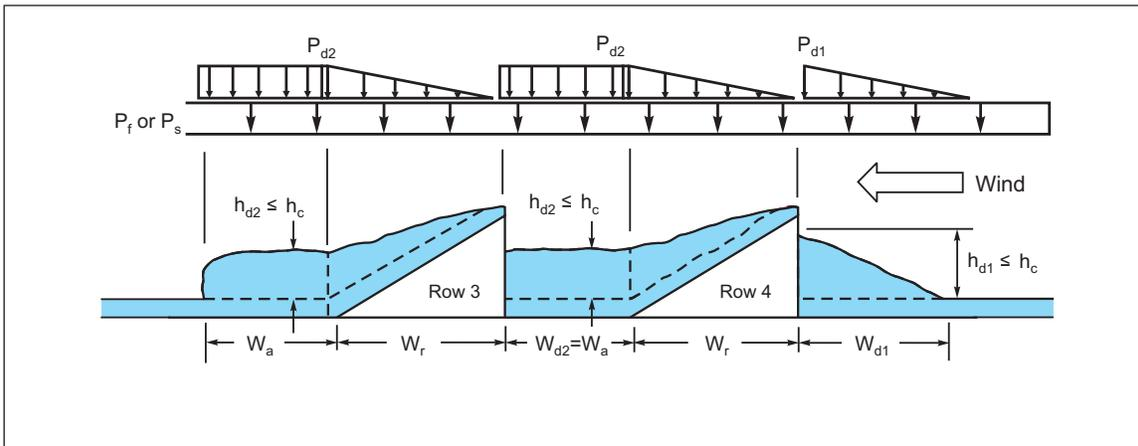
Fig. 2.6.2.3-13. Snow drift loads at tilted solar panel for closely spaced rows with panels facing leeward
