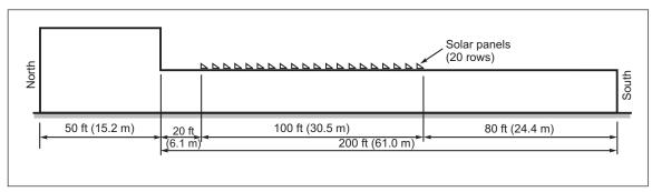
Fig. E.3-2 Elevation view of roof with solar panels
