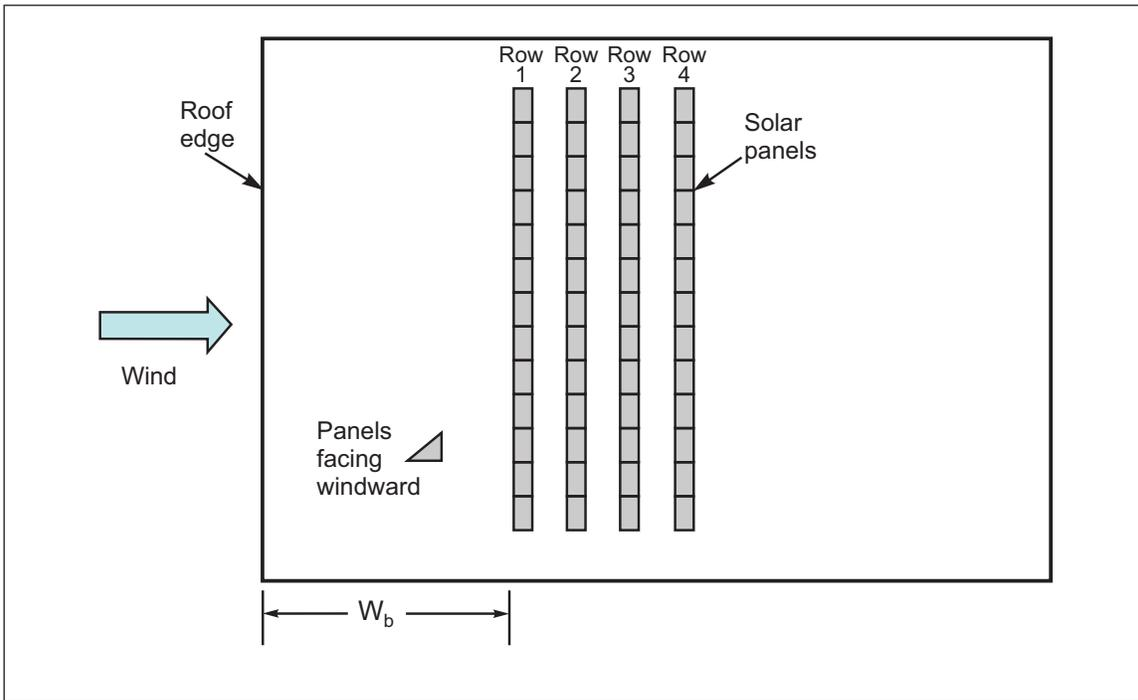
Fig. 2.6.2.3-12. Upwind fetch distance ( $W_b$ ) for snow drift at multiple rows of closely spaced tilted solar panels with panels facing windward
