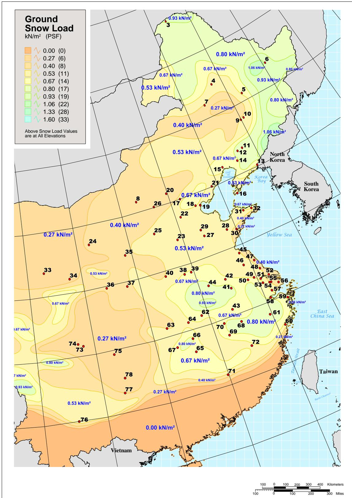
Fig. C4. Ground snow load (Pg) in kN/m<sup>2</sup> for Eastern China
