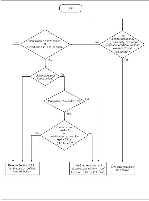
Fig. 2.3.1. Roof live load reduction flow chart
