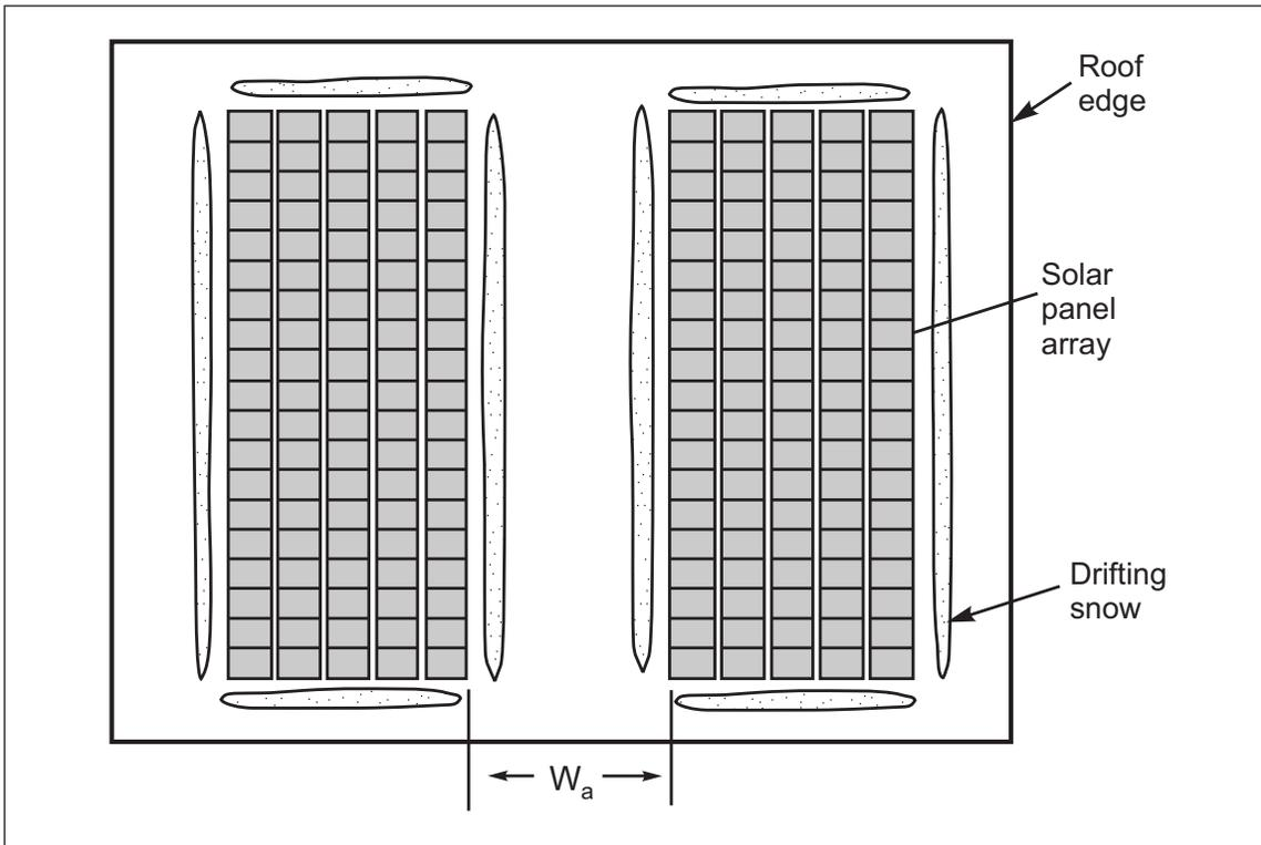
Fig. 2.6.2.3-7. Drifting snow load at flush-mounted solar panel arrays
