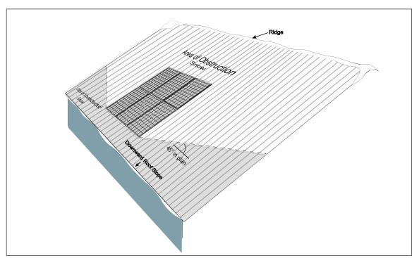
Fig. 2.6.2.3-2. Obstructed portions of sloped roofs
