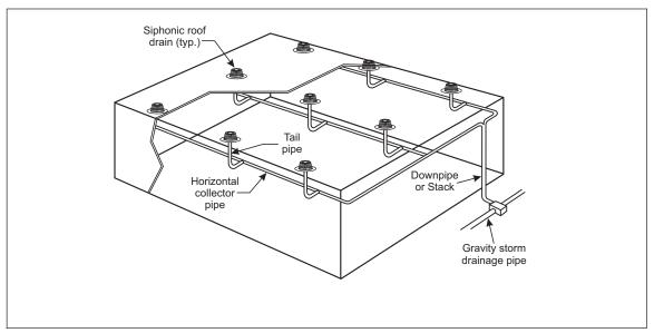
Fig. 2.5.4.2-1. Diagram of siphonic roof drain system
