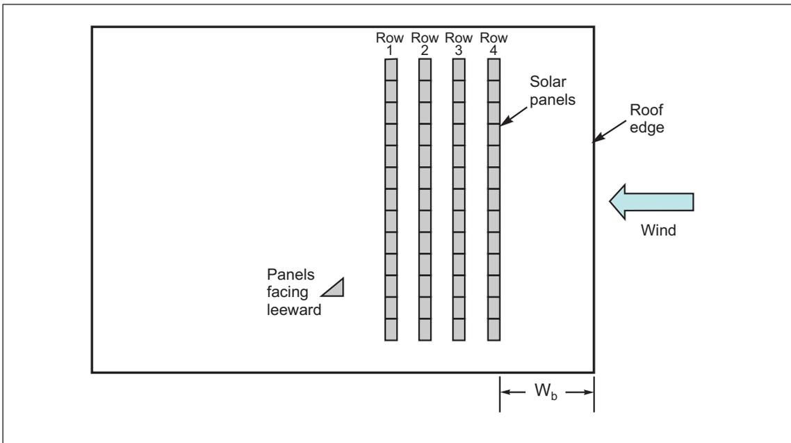
Fig. 2.6.2.3-14. Upwind fetch distance ( $W_b$ ) for snow drift at multiple rows of closely spaced tilted solar panels with panels facing leeward
