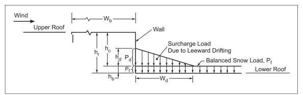
Fig. 2.4.5.1-1. (To be used with Table 2.4.5.1) Leeward snow loads for lower roofs
