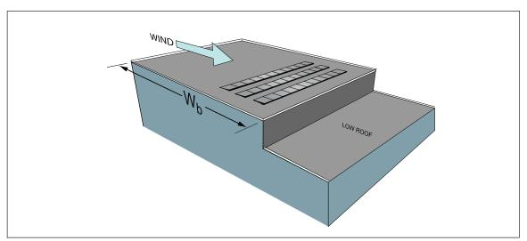
Fig. 2.6.2.3-5. Upwind fetch distance (W<sub>b</sub>) for leeward snow drift at low roof with solar panels on high roof
