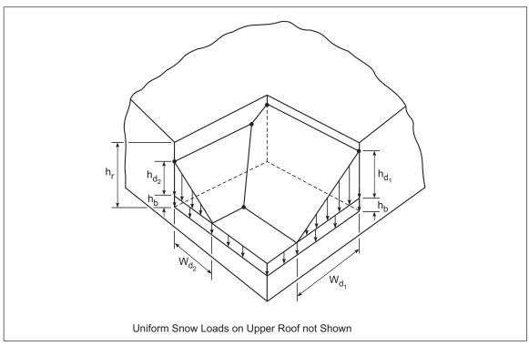
Fig. 2.4.5.1-2. Snow drift intersection at lower roofs
