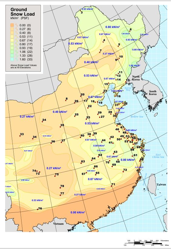
Fig. C4. Ground snow load (Pg) in kN/m<sup>2</sup> for Eastern China
