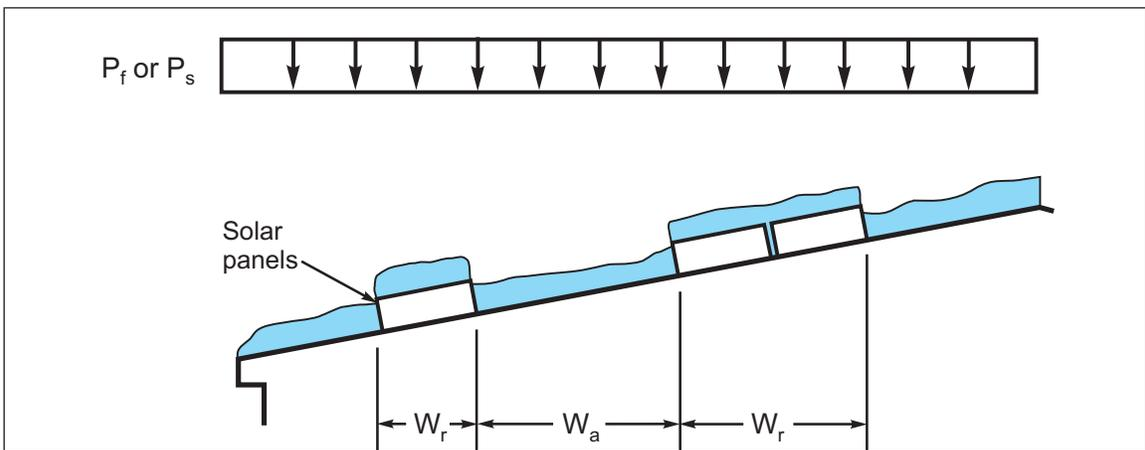
Fig. 2.6.2.3-3. Balanced snow loads on roofs with flush-mounted solar panels
