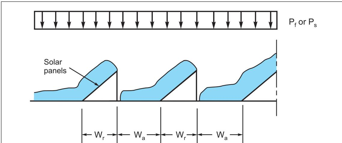
Fig. 2.6.2.3-4. Balanced snow loads on roofs with tilted solar panels
