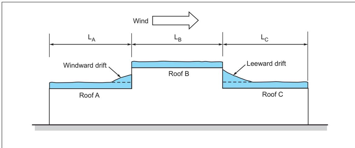
Fig. 3.4. Typical windward and leeward snow drifting
