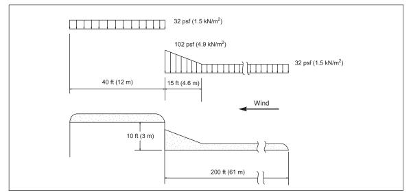
Fig. E.1-4. Design snow loads for Example 4 (Windward Drifting)
