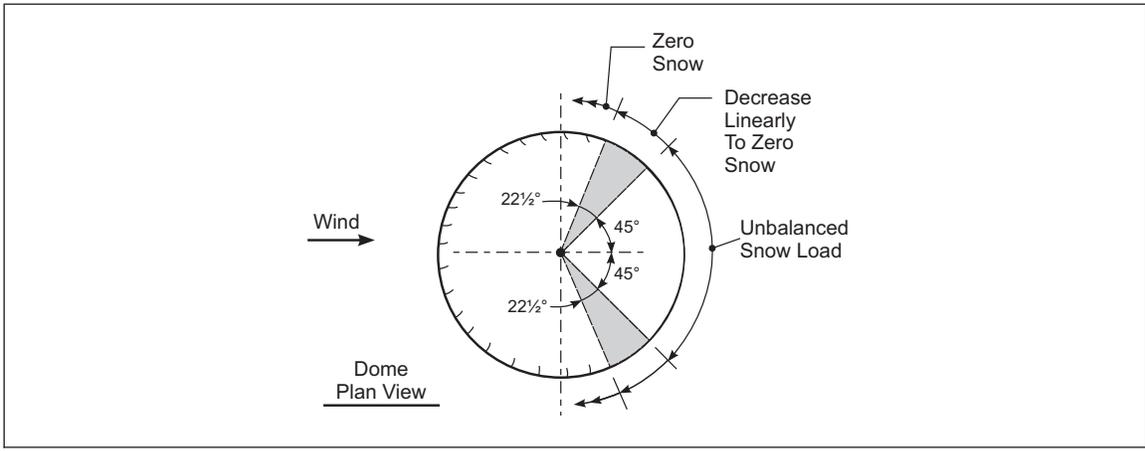
Fig. 2.4.4.4-2. Unbalanced snow load distribution on dome roofs
