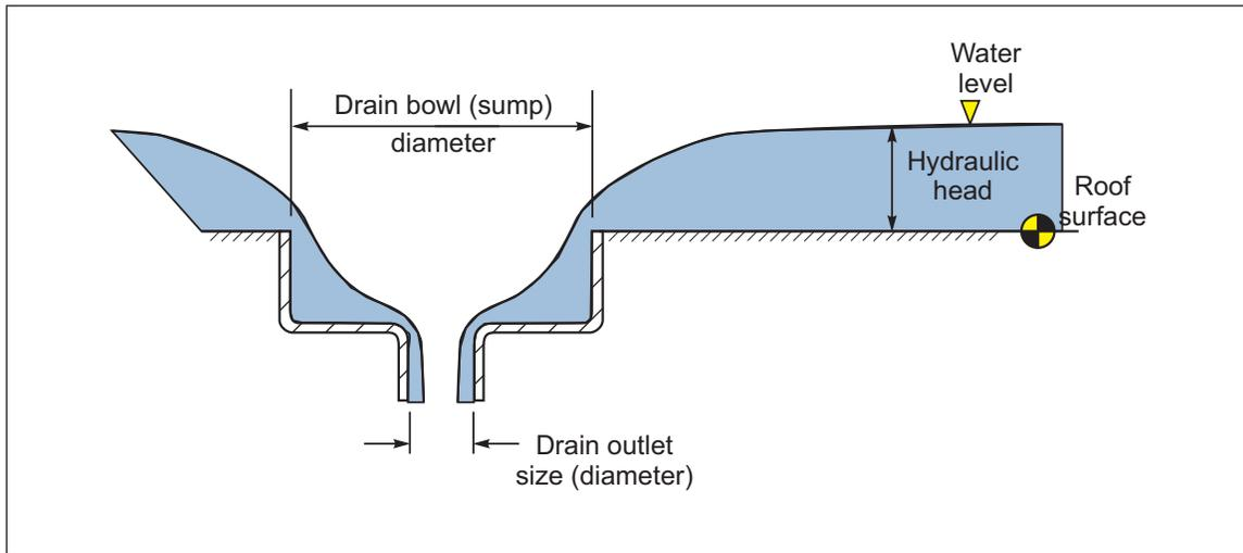
Fig. 2.5.4.1-1. Primary roof drain and hydraulic head (debris guard not shown for clarity)
