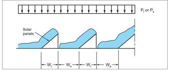
Fig. 2.6.2.3-4. Balanced snow loads on roofs with tilted solar panels
