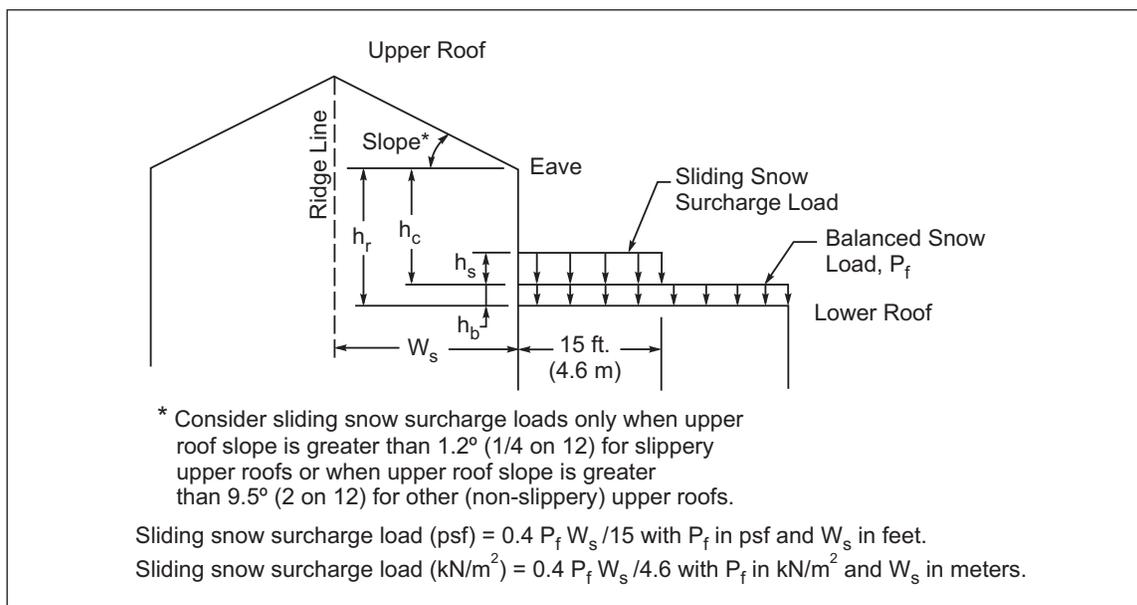
Fig. 2.4.5.2. Sliding snow for lower roofs (upper roof snow load not shown)
