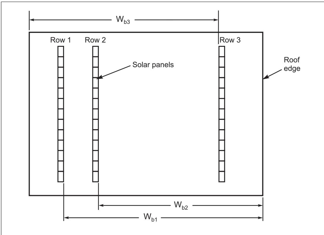
Fig. 2.6.2.3-10. Upwind fetch ( $W_b$ ) for drift load at widely spaced, or single row, solar panels (drifting is not shown)
