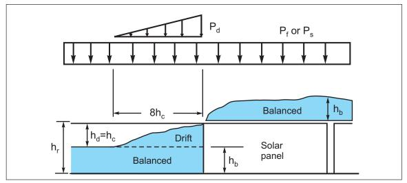
Fig. 2.6.2.3-6. Balanced and drifting snow load at flush-mounted solar panel array
