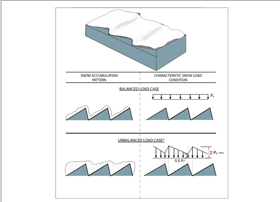
Fig. 2.4.4.5. Snow loads for sawtooth valley roofs
