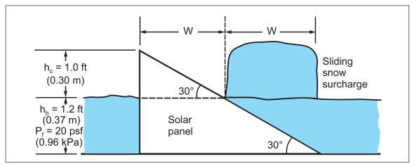
Fig. E.3-4 Sliding snow surcharge load at tilted solar panel
