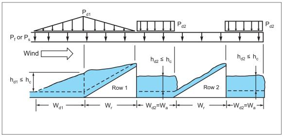
Fig. 2.6.2.3-11. Snow drift loads at tilted solar panels for closely spaced rows with panels facing windward
