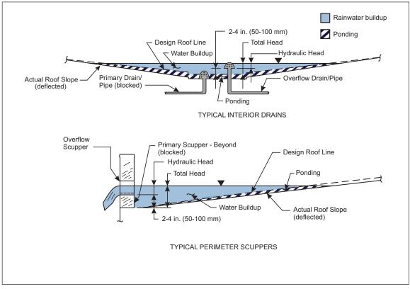
Fig. 2.5.2.1-1. Typical primary and overflow systems for pitched roofs
