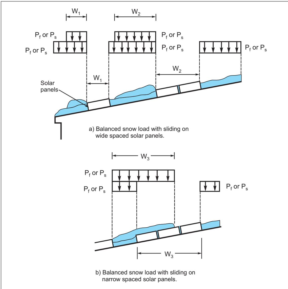
Fig. 2.6.2.3-16. Balanced snow plus sliding snow load with flush-mounted solar panels
