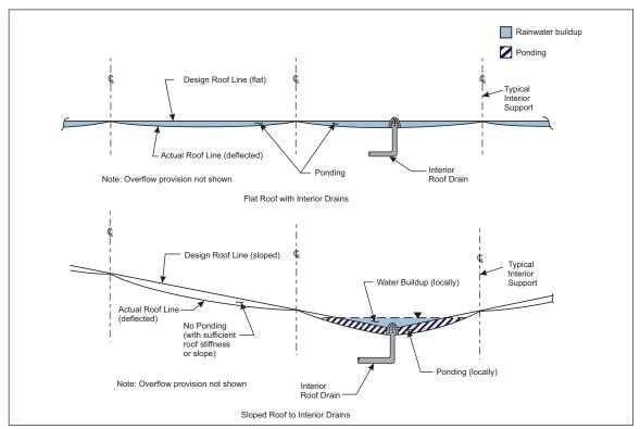
Fig. 2.5.4.1-3. Flat and sloped roofs with interior roof drains
