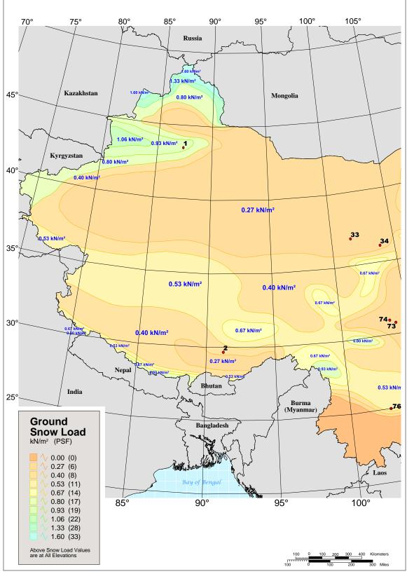
Fig. C3. Ground snow load (Pg) in kN/fm<sup>2</sup> for Western China
