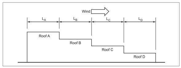
Fig. 2.4.5.1-3. W<sub>b</sub> for leeward snow drift at multiple roofs steps
