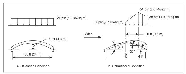
Fig. E.1-2. Design snow loads for Example 2
