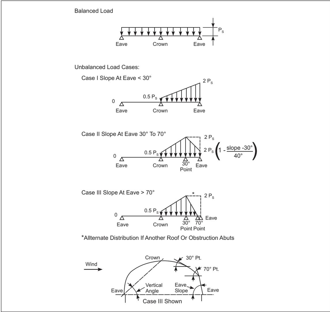
Fig. 2.4.4.4-1. Snow loads for curved and dome roofs
