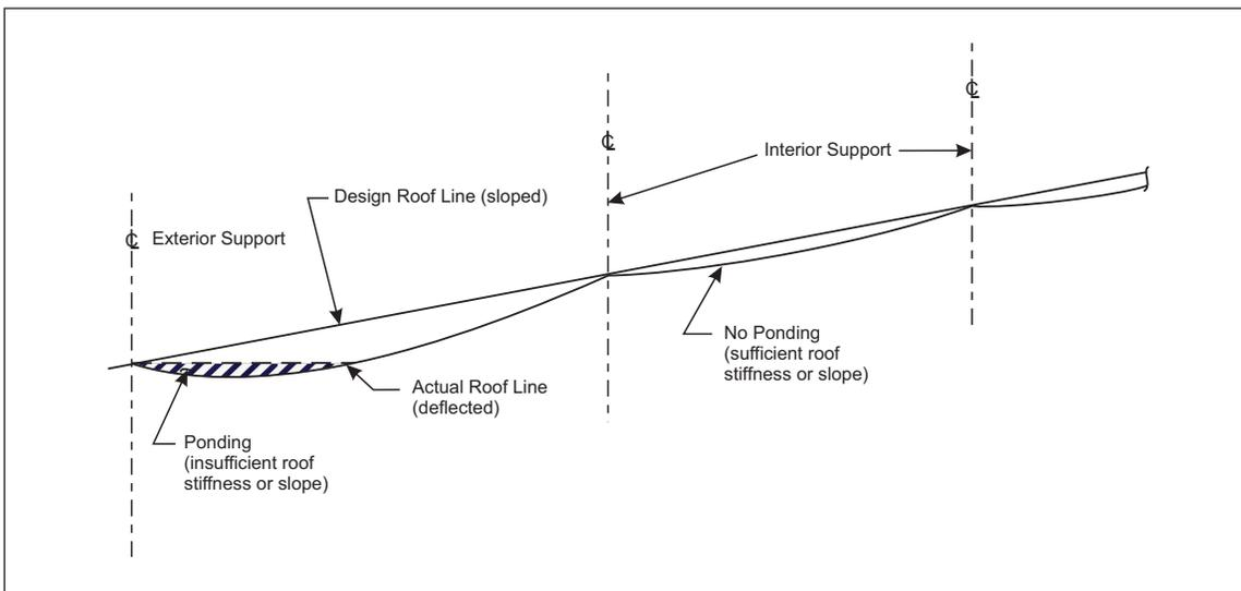
Fig. 2.5.4.1-4. Sloped roof with roof edge drainage
