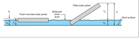
Fig. 2.6.2.3-1. Flush-mounted and tilted solar panels, schematic elevation view
