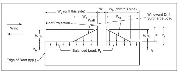
Fig. 2.4.5.1-5. Snow load at roof projections
