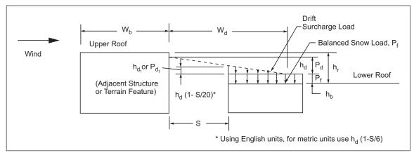
Fig. 2.4.5.1-4. Snow loads for lower roof of adjacent structures
