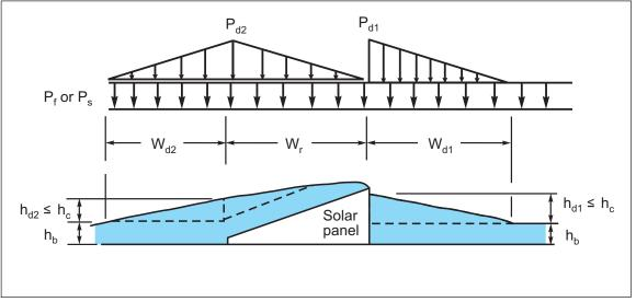
Fig. 2.6.2.3-9. Snow drift loads at tilted closed-back solar panel widely spaced rows (or a single row)
