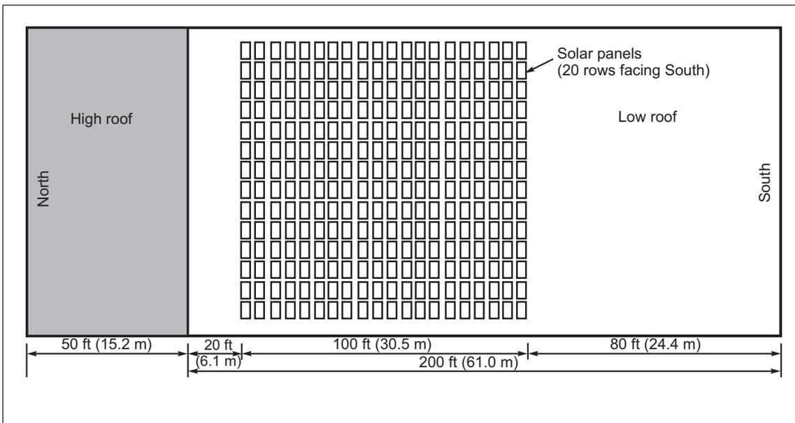
Fig. E.3-1 Plan View of Roof with solar panels
