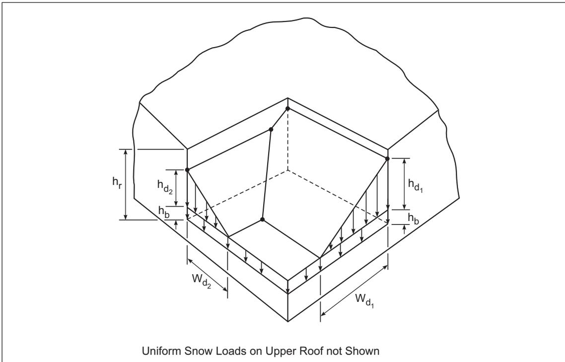
Fig. 2.4.5.1-2. Snow drift intersection at lower roofs
