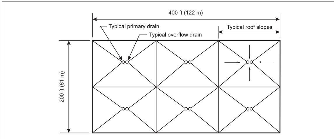
Fig. E.2-3. Roof plan for Example 6
