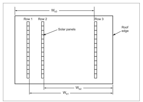
Fig. 2.6.2.3-10. Upwind fetch  $(W_b)$  for drift load at widely spaced, or single row, solar panels (drifting is not shown)
