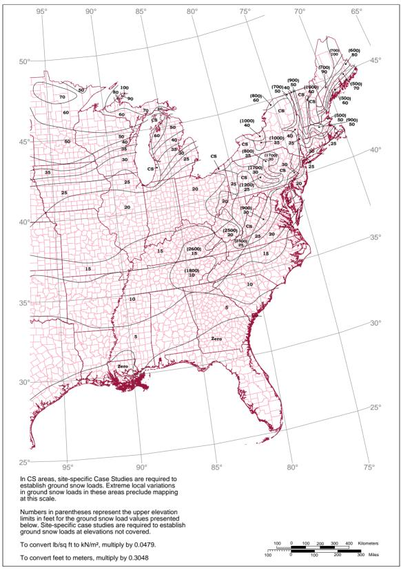
Fig. C2. Ground snow load (Pg) in psf for eastern United states (to obtain kN/m2, multiply by 0.048)
