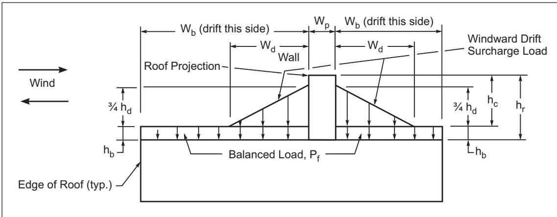
Fig. 2.4.5.1-5. Snow load at roof projections
