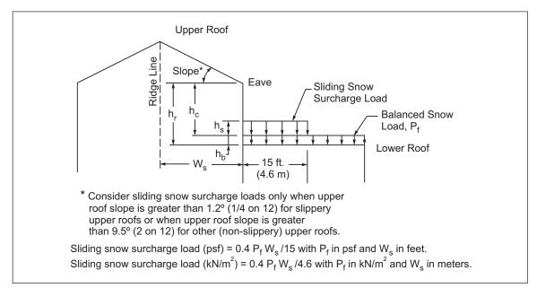
Fig. 2.4.5.2. Sliding snow for lower roofs (upper roof snow load not shown)
