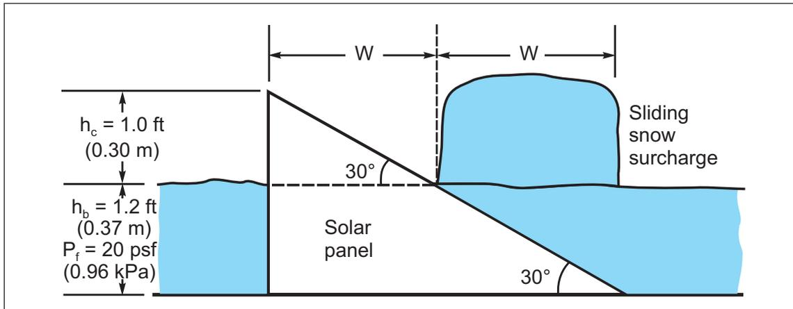
Fig. E.3-4 Sliding snow surcharge load at tilted solar panel
