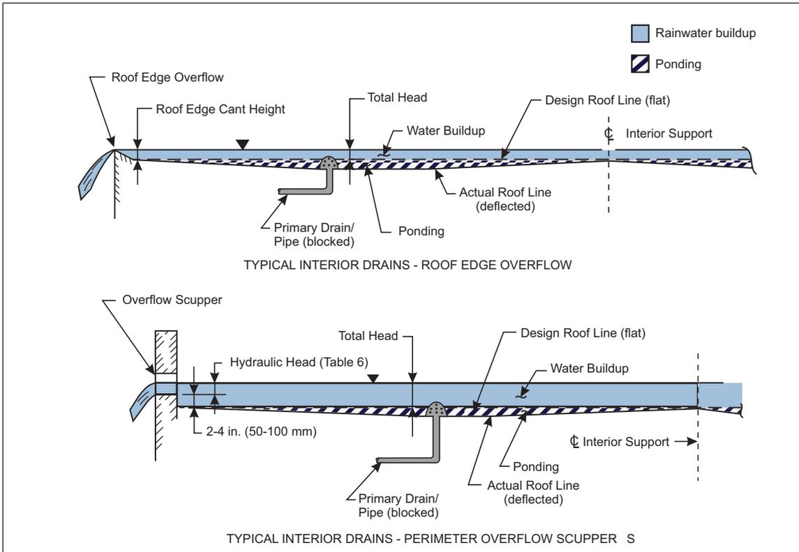
Fig. 2.5.2.1-2. Typical primary and overflow drainage systems for flat roofs
