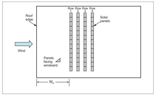
Fig. 2.6.2.3-12. Upwind fetch distance (W<sub>b</sub>) for snow drift at multiple rows of closely spaced tilted solar panels with panels facing windward
