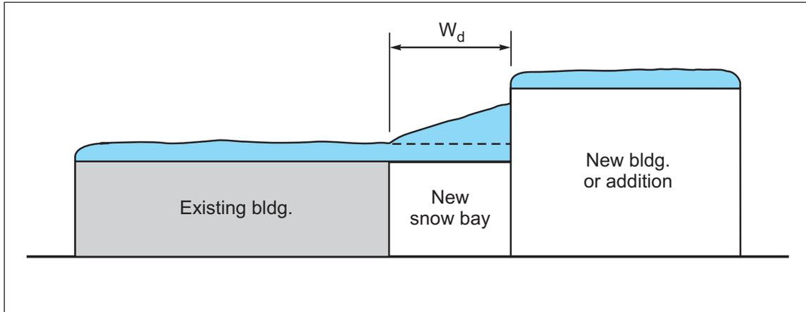
Fig. 2.4.6. New snow bay to prevent drift loading on an existing roof
