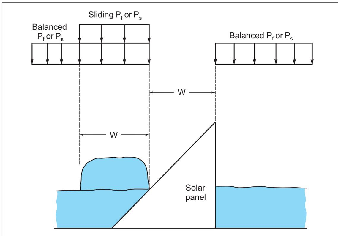
Fig. 2.6.2.3-17. Sliding snow load at tilted solar panels
