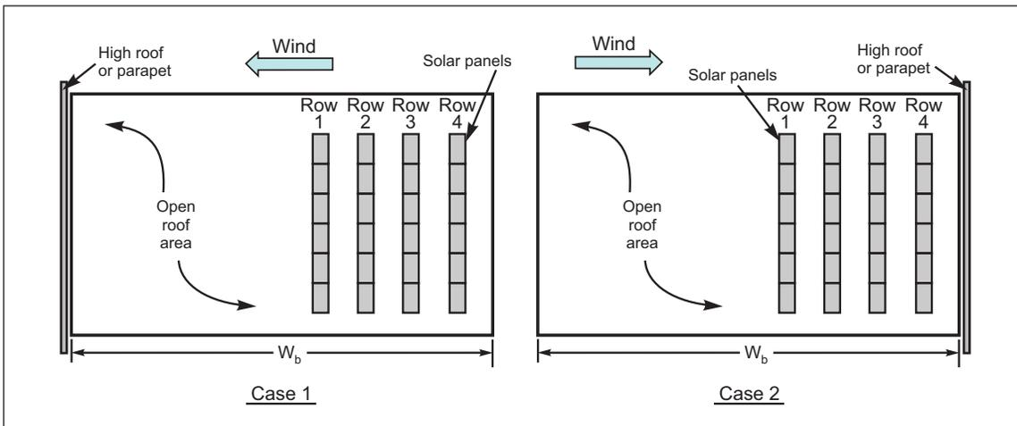
Fig. 2.6.2.3-8.  $W_b$  for snow drift at parapets, roof projections, or high roof walls for flush-mounted solar panels, widely-spaced tilted solar panels, and tilted solar panels with less than significant height
