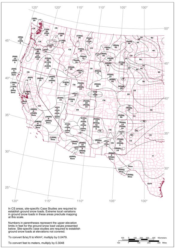
Fig. C1. Ground snow load (Pg) in psf for western United States
